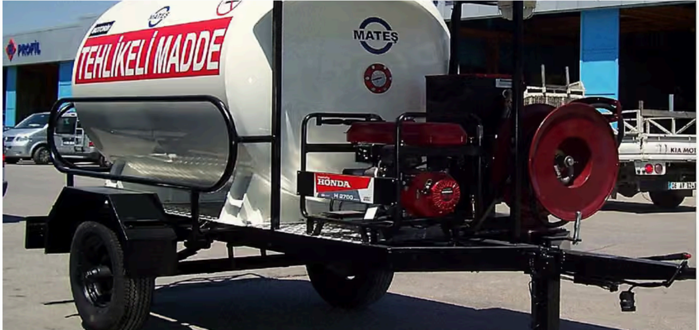
Fig. 1 · MATES mobile refuelling trailer with canopy, hose reel and pump, outdoors at the plant. Livery and equipment vary per order.
