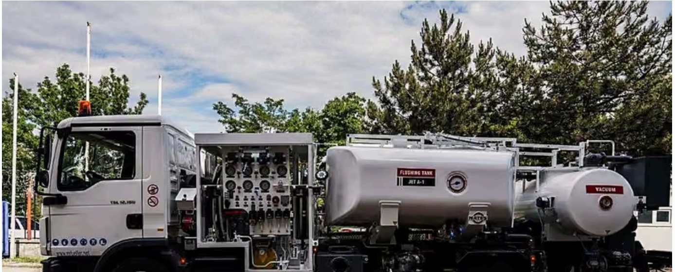
Fig. 1 · MATEŞ hydrant pit cleaner in side profile with its equipment cabinet open. Livery and equipment vary per order.
